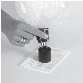
Separating valve and filling chamber
