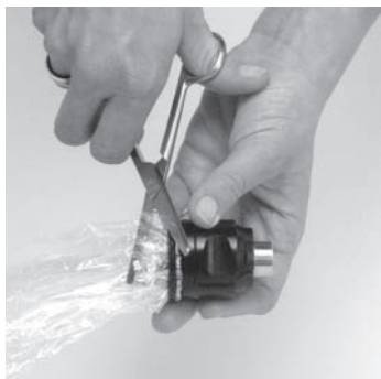
Trimming the excess of the oven tube
